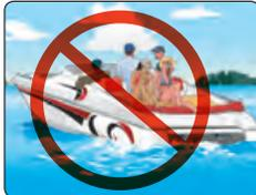
The operator must limit the vessel’s load to the total weight or maximum number of persons shown on the capacity plate, whichever is more restrictive.
